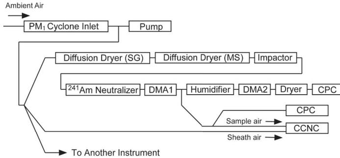
**Fig. 1.** Schematic diagram depicting the instrumental arrangement used for atmospheric measurements (HTDMA coupled to the CCNC). The instrument was used for the observation of this project until 1 April 2008, and that after 3 April in a related research project. Modified from Mochida *et al.* (2010) by permission of American Geophysical Union (AGU). Copyright 2010 AGU.
