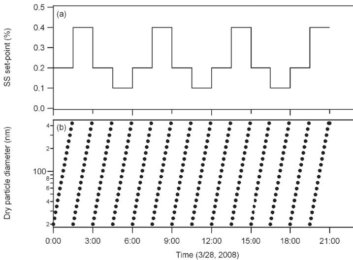
**Fig. 2.** Example of (a) the setting of the CCNC and (b) the dry mobility diameter setting of DMA1 in the HTDMA, for observations conducted at Cape Hedo, Okinawa, on 28 March 2008. The HTDMA data collected for diameters of 24.1–359 nm were used for the analyses. The CCNC were operated in collaboration with related research projects. The collected CCNC data have not been analyzed for the characterization of the CCN activity.
