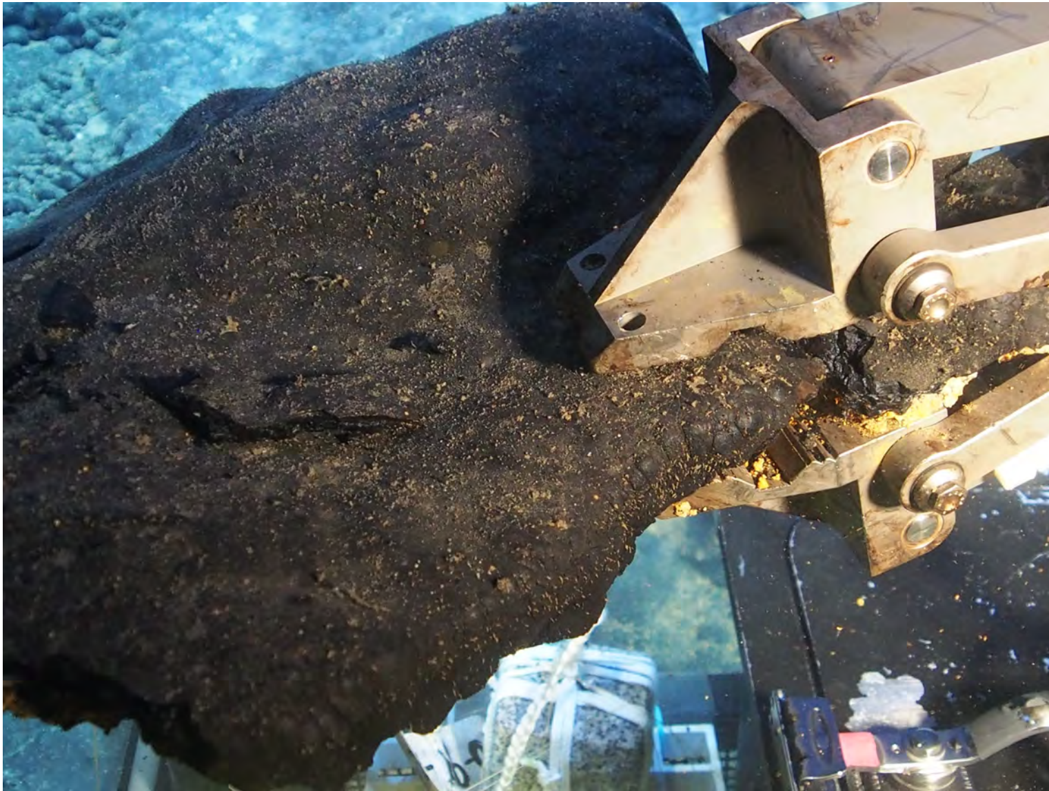
Fig. S1. Sampling photo of KAIKO#684-R05 at 4441 m depths using a manipulator of ROV Kaiko deployed from RV Kairei .
