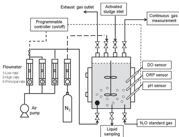
Fig. 1. Schematic of the laboratory-scale incubation reactor.
