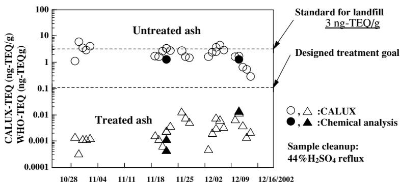
Fig. 1. Dioxin monitoring results during the Hagenmaier process at one actual plant using DR-CALUX and chemical analysis.
