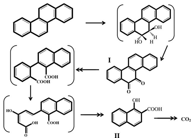
Fig. 3. A proposed pathway for the degradation of chrysene by *Polyporus* sp. S133. Compounds in brackets were not identified in our culture extracts.
