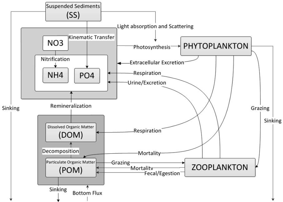
Fig. 1. Schematic diagram of marine ecosystem model. The model has 8 compartment biological tracers. The arrows indicate nitrogen flow among biological tracers.
