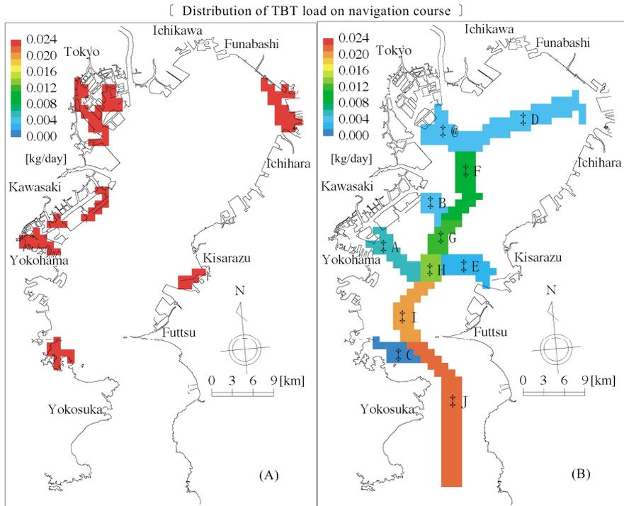
Fig. 2. Estimate of the distribution of TBT load along navigation routes and in ports of Tokyo Bay. (A): Distribution within each port, and (B): distribution along shipping navigation course.
