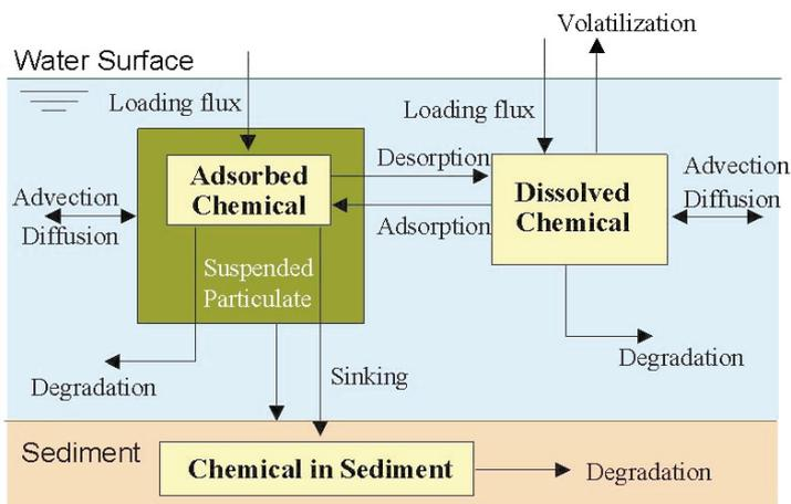
Fig. 1. Model concept for predicting the fate of a chemical contaminant.
