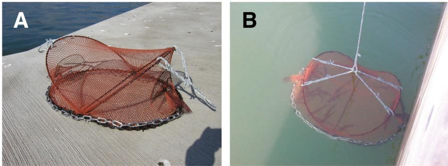
Fig. 2. Photographs of the cage used for immersion survey. A: an external form of cage, B: suspended and immersed cage in the survey site.
